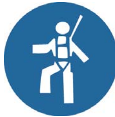
Compulsory personal protection against falls
